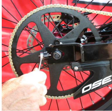
Chain tensioner nut (10mm).
